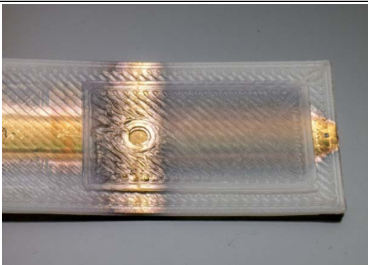
Printed polymer/gold structure with via-contact and track access
