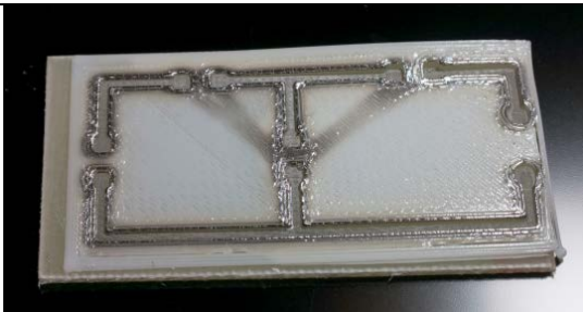
Printed polymer mask on FR4, metallised and reinforced by galvanic
